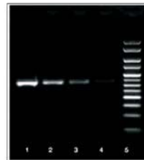
High performance with PANScript A 175 bp fragment was amplified from pG EM 3z f(+) using PANScript DNA-Polymerase. Lane 1 - 4: 10-fold serial dilution of template. (starting concentration 25 ng/µl) Lane 5: PANLadder V
