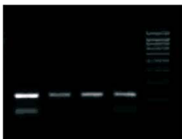
Lane 1: PCR mix before cleaning, 125 bp fragment Lane 2: PCR mix treated with PAN DNA Clean 1:1 Lane 3: PCR mix treated with PAN DNA Clean 1:2 Lane 4: Purification with PCR Clean up Kit (Silica membrane) Lane 5: PANLadder I
